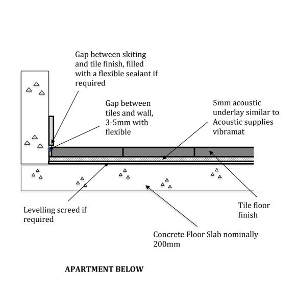
Tiled Hard Floor Finished within Habitable areas Acoustic Treatment Lntw + C1 < 62 and IIC 50
