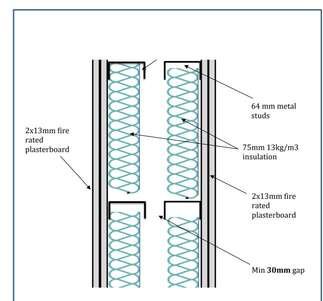
NOTE: All junctions between the plasterboard and the building structure to be sealed using a 10-20mm gap filled with a flexible acoustic sealant.
