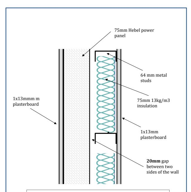
NOTE: All junctions between the plasterboard, Hebel and the building structure to be sealed as required by the CSR specifications.
